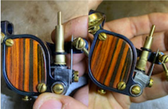
**IL EST DE MÊME FORTEMENT DÉCONSEILLÉ DE TROP COMPRESSER LE RESSORT EN TOURNANT DANS LE SENS DES AIGUILLES D'UNE MONTRE, CE QUI AURAIT POUR EFFET D'ÉCRASER LE RESSORT DÉFINITIVEMENT ET NUIRE AU FONCTIONNEMENT DE LA MACHINE.**
